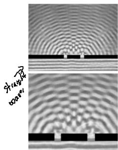
here is a diagram of a double slit interference pattern notice the straight waves approaching the barrier from the bottom
