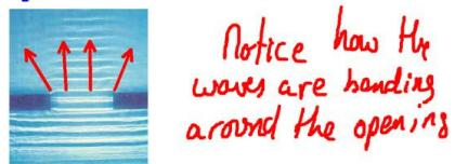
Notice how the waves are bending around the opening
